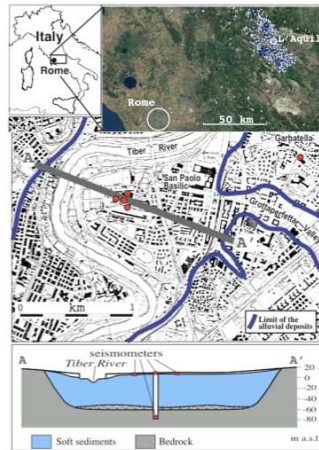
Figure 1: Top panel: epicenter of L'Aquila 6th April 2009 M_w=6.1 damaging earthquake with the epicenters of the seismic sequence. Middle panel: 3D array location, red spots represent seismic stations. The red spot outside the Tiber valley (Garbatella) is the reference station. Bottom panel: sketch of the borehole station located beneath the alluvial sediments layer. See paper P2 for details.
