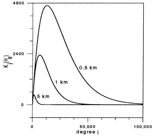
Fig. 1. Transfer function  $K_j(H_0)$  between unknown coefficients  $T_{jm}$  and gravity anomalies  $\Delta g^h$  for  $H_0 = 1$  km, 5 km, and 10 km
