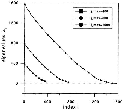
**Fig. 4.** The eigenvalue spectra of matrix  $A$  for various cut-off degrees  $j_{max}$  and a body with axisymmetric surface generated by height  $H(\vartheta, \lambda = 80^\circ)$  multiplied by 10 ( $j_{min} = 21$ ). The ellipsoidal corrections  $\epsilon_h$  and  $\epsilon_\gamma$  are equal to zero
