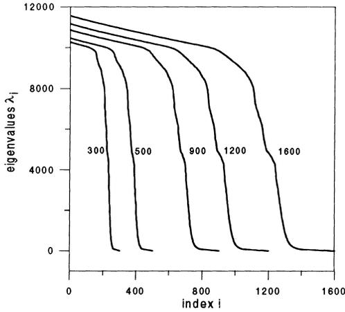
**Fig. 6.** The eigenvalue spectra of matrix  $A$  for various cut-off degrees  $j_{max} = j_{min} + \Delta j$ ,  $\Delta j = 300, 500, \dots, 1600$ , and a body with axisymmetric surface generated by height  $H(\vartheta, \lambda = 80^\circ)$  ( $e_0^2 = 0$  and  $j_{min} = 10\,000$ )
