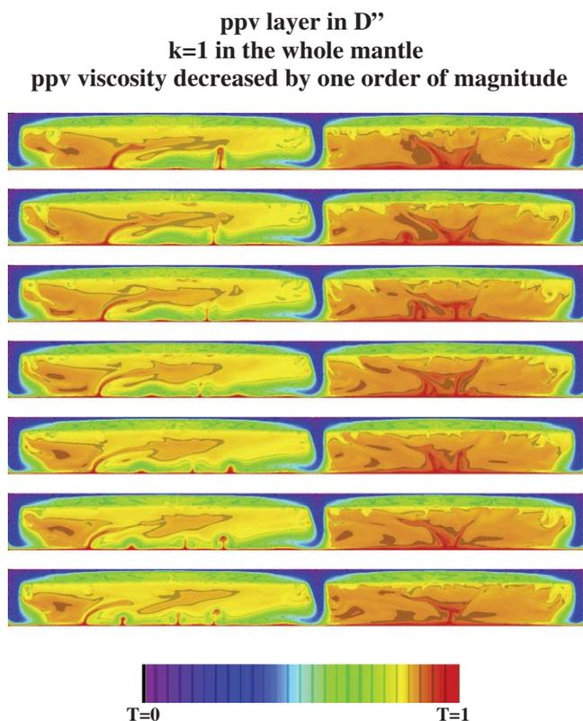
**Fig. 5.** Snapshots of the dimensionless temperature field for a model with the same  $G(z)$  as in Fig. 2 and with a perovskite to postperovskite phase change. Thermal conductivity is constant throughout the whole mantle. The viscosity is decreased by a factor of 10 in ppv.
