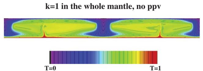
**Fig. 2.** One snapshot of the dimensionless temperature field for the model with activation energy  $G(z)$  shown in Eq. (4), with constant thermal conductivity and without ppv phase transition.
