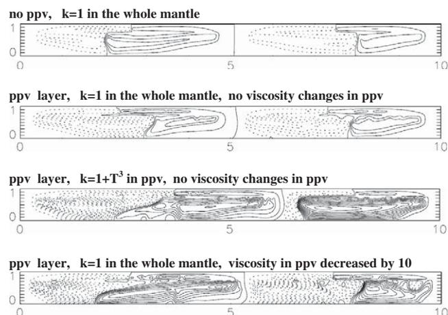
**Fig. 6.** Stream function for the models shown in Figs 2–5. Solid lines correspond to clock-wise motion, dashed lines indicate anti-clock-wise motion. We call attention to the complex multiscale circulatory patterns in the bottom two panels in contrast to the topmost panel.
