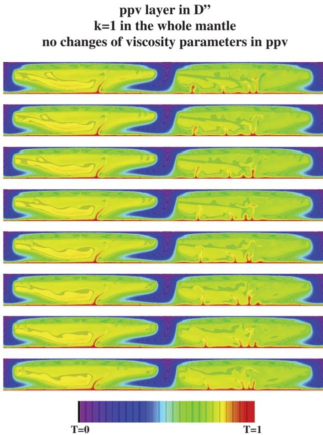
**Fig. 3.** The dimensionless temperature field for a model with the same  $G(z)$  as in Fig. 2 and with a perovskite to postperovskite phase change. Thermal conductivity is constant throughout the whole mantle.
