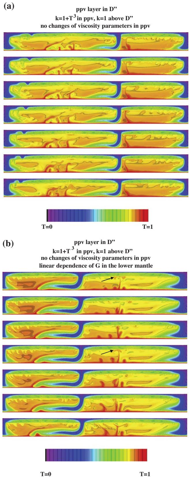
**Fig. 4.** (a) Snapshots of the dimensionless temperature field for a model with the same  $G(z)$  as in Fig. 2, with a perovskite to postperovskite phase change and a temperature-dependent thermal conductivity in ppv. (b) The same, but now for linearly increasing  $G(z)$ . Black arrows indicate the positions of the hot anomalies below the 670 km boundary.
