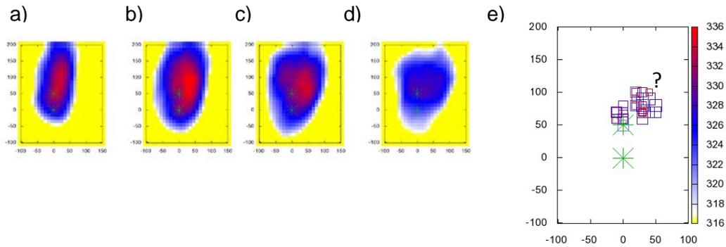
**Figure. S4.** Back-projection of regional waveforms of Event 2. Analogous to Fig. S3. Panels **a) - d)** show the temporal evolution of the brightness in a NS-EW kilometric grid at 8, 10, 12, and 14 s after hypocentre time, respectively. Epicentres of Event 1 and 2 are shown by asterisks. **e)** Maximum brightness  $B_{max}$  at each computed time slice; time is measured with respect to origin time of Event 1 (time 0). The question mark shows limited reliability of the NE patch.
