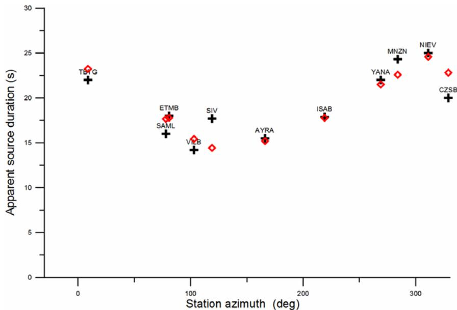
**Figure S1.** Directivity of Event 1. The azimuthal variation of the apparent source duration (crosses) is in agreement with a unilateral model (diamonds).
