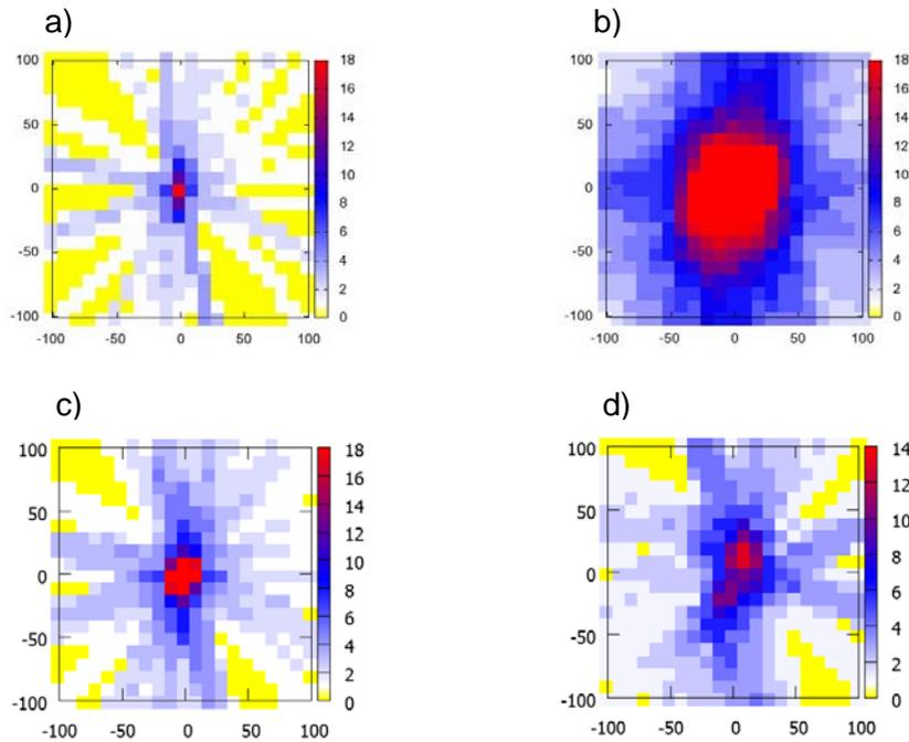
**Figure S2.** Synthetic modelling the back-projection for a point source in a NS-EW, 200x200 km grid. In panels **a)** and **b)** the back-projection makes use of the correct source depth, assuming temporal error of  $\pm 0.5$  and  $\pm 3$  seconds, respectively. In panels **c)** and **d)** the back-projection assumes a temporal error of  $\pm 1$  s and makes use of correct depth in panel c and an incorrect depth (20 km shallower) in panel d.
