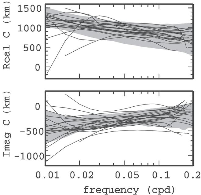
**Figure 2.** The Schumaker  $C$ -responses generated by the 3-D conductivity model. At middle geomagnetic latitudes,  $25^\circ \leq |\lambda_d| \leq 65^\circ$ , these are limited to the areas shown by grey shading. Local 1-D responses computed by *Schultz and Larsen* [1987] for 22 ground stations are stacked over using solid lines.
