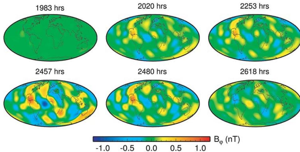
**Figure 4.** The computed  $B_\phi$  component at satellite altitude 400 km. Snapshot at  $t = 1983$  h corresponds to the onset of the magnetic storm. At  $t = 2020$ , and 2457 h the storm culminates, and  $t = 2253$ , 2480, and 2618 h sample the recovery phases. The time snapshots are marked in Figure 3
