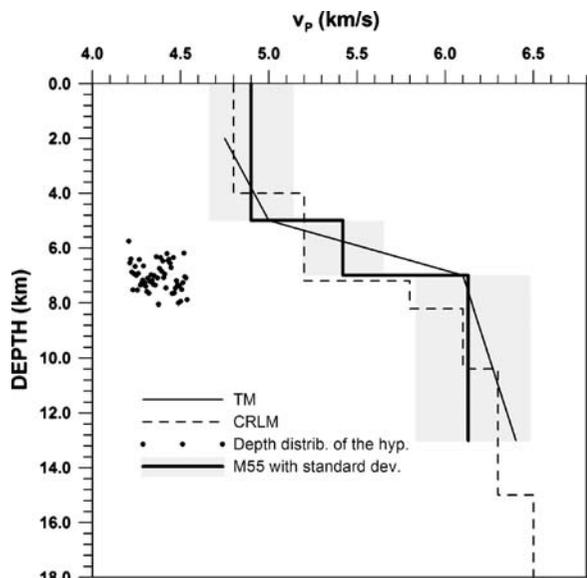
**Fig. 4**  $P$ -wave velocities in the individual layers of the M55 model, derived in the present study (solid line). The shaded zone gives their standard deviation obtained by delete-one jackknifing. The average tomography model TM and the CRLM model are shown for comparison. The group of dots represent the depth distribution of the hypocentres of events, located by the HYPO code in the CRLM model (The coordinate in the horizontal axis for dots is arbitrary)
