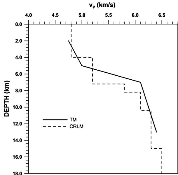
**Fig. 2** 1-D velocity models: TM is the average model from tomography for subregions a) and b) shown in Fig. 1. CRLM is the model used for HYPO locations by the Corinth Rift Laboratory (Rigo et al. 1996)
