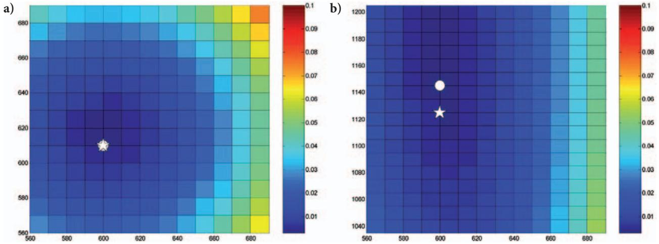
Figure 3 X-Y at Z=1125 m (a), and X-Z at Y=610 m (b) cross-sections of misfit value (sec<sup>2</sup>) of the location of the source, respectively. The inversion uses the surface receivers travel-time data for the true forward model. The asterisk gives the position of the forward source, the circle the position of found hypocentre.
