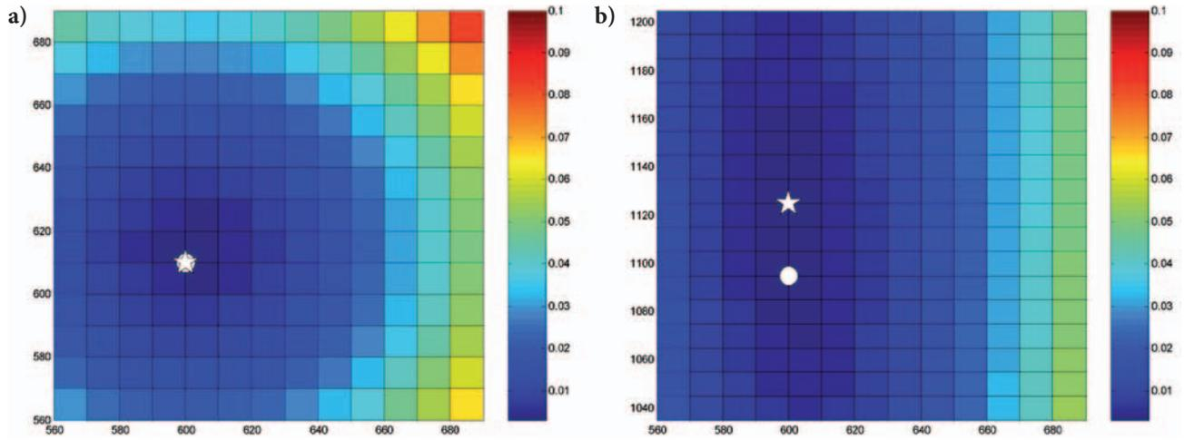
Figure 6 The same as in Figure 3, but for inversion that uses the surface receivers travel-time data for the perturbed forward model. The X–Y crosssection is taken at Z=1095 m. The X–Z crosssection stays at Y= 610 m.
