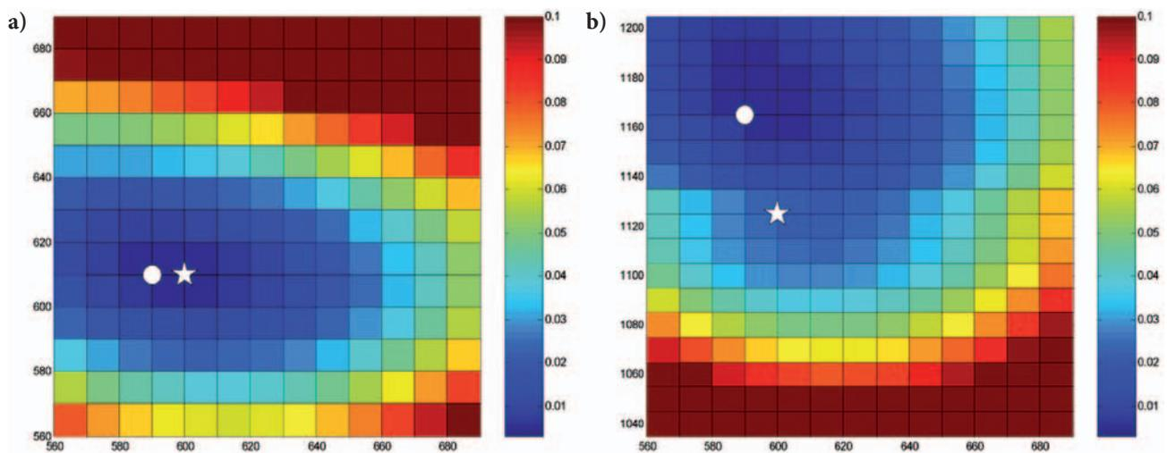
Figure 8 The same as in Figure 5, but for inversion that uses the travel-time data for the perturbed forward model. The X–Y crosssection is taken at Z=1065 m and the X–Z crosssection is taken at Y=610m. The asterisk in Figures 6a, 7a, 7b, and 8a is projected from its proper position.
