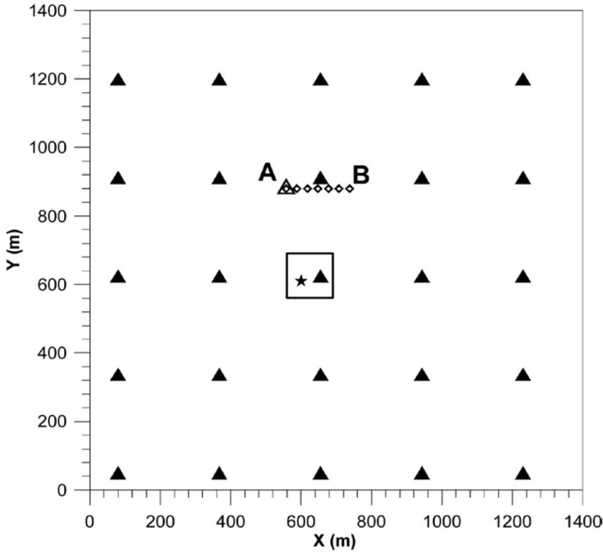
**Figure 2a** Map view of the positions of vertical A (white triangle) and horizontal B (white diamonds) monitoring wells, and of surface receivers network (black triangles). Asterisk denotes the X-Y coordinate of synthetic microseismic event (source point in the model). The rectangle shows the X-Y area of grid, in which we evaluate the misfit value.
