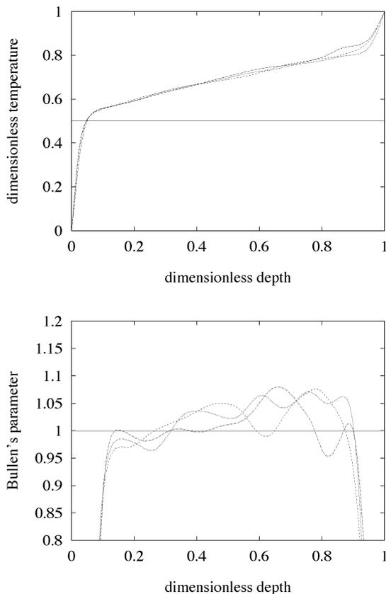
Fig. 4. Three snapshots of dimensionless horizontally averaged temperature  $\langle T \rangle$  and the Bullen parameter  $\eta$  as a function of dimensionless depth  $z$  for the variable thermal conductivity  $k$ , see Eq. 4, constant thermal expansivity  $\alpha=1$  and internal heating  $R=8$ . Otherwise, same as in Fig. 1.
