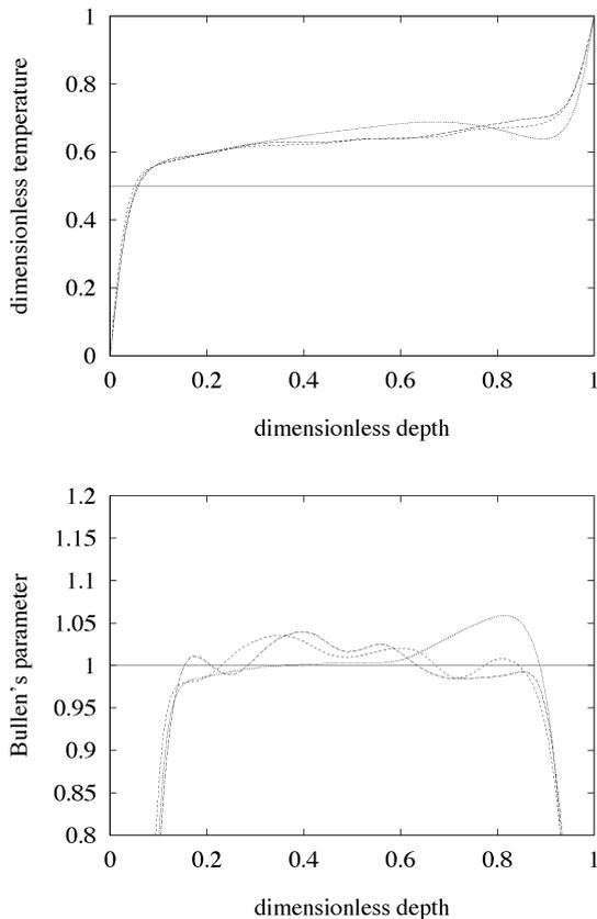
Fig. 6. Three snapshots of dimensionless horizontally averaged temperature  $\langle T \rangle$  and the Bullen parameter  $\eta$  as a function of dimensionless depth  $z$  for the constant thermal conductivity  $k=1$ , depth-dependent thermal expansivity  $\alpha(z)$ , see Eq. 5, and internal heating  $R=8$ . Otherwise, same as in Fig. 1.
