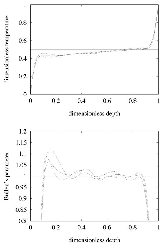
Fig. 5. Three snapshots of dimensionless horizontally averaged temperature  $\langle T \rangle$  and the Bullen parameter  $\eta$  as a function of dimensionless depth  $z$  for the constant thermal conductivity  $k=1$ , depth-dependent thermal expansivity  $\alpha(z)$ , see Eq. 5, and purely basal heating  $R=0$ . Otherwise, same as in Fig. 1.
