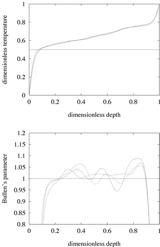
Fig. 2. Three snapshots of dimensionless horizontally averaged temperature  $\langle T \rangle$  and the Bullen parameter  $\eta$  as a function of dimensionless depth  $z$  for the constant thermal conductivity  $k=1$ , constant thermal expansivity  $\alpha=1$  and internal heating  $R=8$ . Otherwise, same as in Fig. 1.
