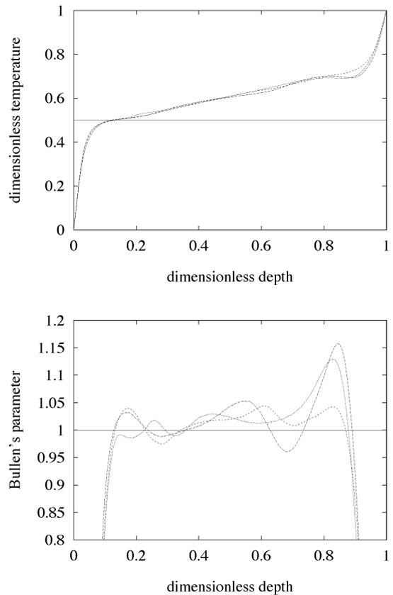
Fig. 3. Three snapshots of dimensionless horizontally averaged temperature  $\langle T \rangle$  and the Bullen parameter  $\eta$  as a function of dimensionless depth  $z$  for the variable thermal conductivity  $k$ , see Eq. 4, constant thermal expansivity  $\alpha=1$  and purely basal heating  $R=0$ . Otherwise, same as in Fig. 1.
