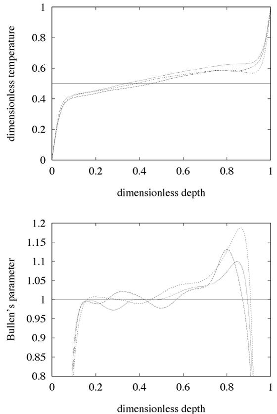
Fig. 1. Three snapshots of dimensionless horizontally averaged temperature  $\langle T \rangle$  and the Bullen parameter  $\eta$  as a function of dimensionless depth  $z$  for the constant thermal conductivity  $k=1$ , constant thermal expansivity  $\alpha=1$  and purely basal heating  $R=0$ . To obtain  $\eta(z)$  we averaged  $dT/dz$  and  $T$  over the interval  $\langle z-0.05, z+0.05 \rangle$ , which corresponds to 300 km in the Earth's mantle.
