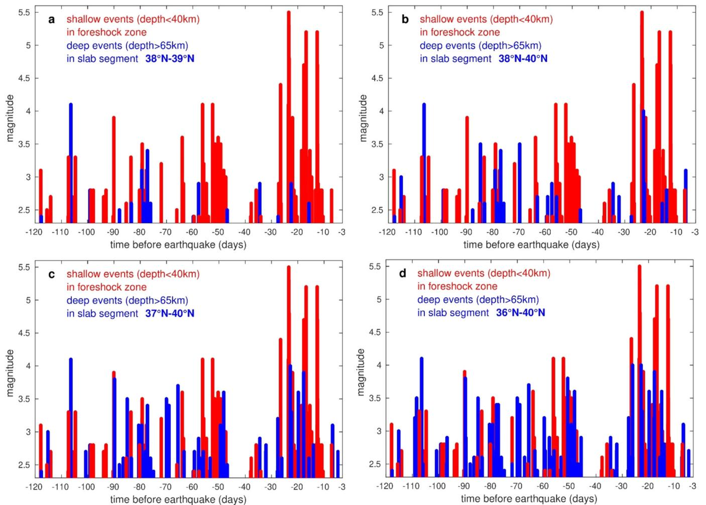
**Fig. 5.** Comparison of the timings of shallow events in the foreshock/epicentral zone (a circle of 75 km around the epicenter) with events occurring deep in the slab in the 4 months preceding the Tohoku earthquake. The slab section considered for the deep activity increases from (a) to (d) and is indicated in each panel. As the length of the slab section increases, a synchronization emerges between the two activities.
