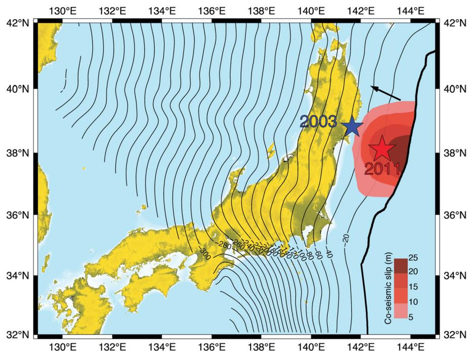
**Fig. 7.** Locations of the largest intermediate-depth earthquake (M7.1 in blue) and the largest subduction earthquake (M9.0 in red) in instrumental time in Honshu. The Tohoku coseismic slip determined from the inversion of GPS data by Perfettini and Avouac (2014) is shown in reddish colors. Contour lines show slab interface depth (Hayes et al., 2012). The thick black line is the trench. Arrow indicates the direction of slab descent.
